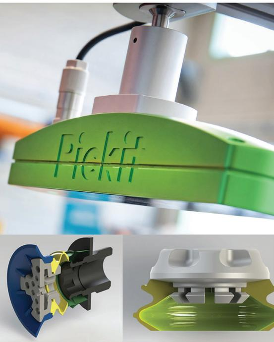
'Pickit 3D' is a plug & play camera that gives robots eyes to enable automation of the 'pick & place-process' in a production line.
